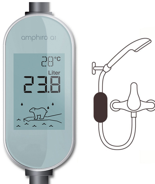
Figure 1: The feedback and measurement device used in this study. Notes. On the left: a snapshot of the feedback displayed by the smart shower meter. On the right: the device installed between the showerhead and shower hose.
